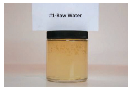
Fig. 2—An initial sample of flowback water from a northern Colorado well contained from 5,000 mg/L to 6,000 mg/L guar.
