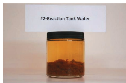
Fig. 3—A water sample showing the effect of the addition of ferric chloride to the reaction tank. A flock was formed and the resulting sludge required removal by a strainer.
