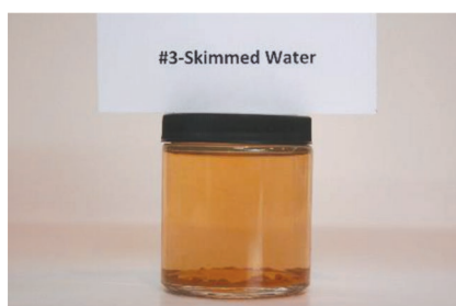
Fig. 4—After the skimming operation, the water was colored slightly orange by the ferric chloride and showed residual suspended solids that settled in the water.
