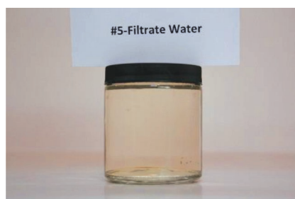
Fig. 6 —After the pH and oxygen reduction potential were adjusted, the water was processed through a crossflow microfiltration system.
